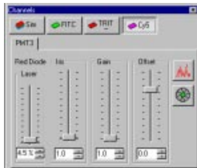
Figure 25 Channels window of Control Panel, Third Sequential Setting button depressed
